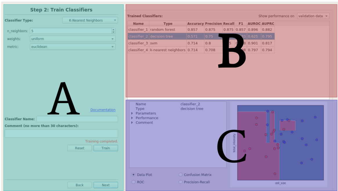
Figure 4.2: The layout of the ml4bio software, with colored panels showing its main sections. Users navigate a machine learning workflow in panel A, view summarized results in panel B, and view detailed information and data visualizations in panel C.
